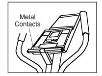
must be touching the lower contacts. Avoid moving your hands. After a moment, the heart-shaped indicator in the display will begin to flash and your heart rate will be shown. For the most accurate heart rate reading, continue to hold the contacts for about 15 seconds.
